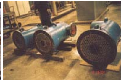
Ingersoll-Rand CENTAC® COOLER REPAIRS
